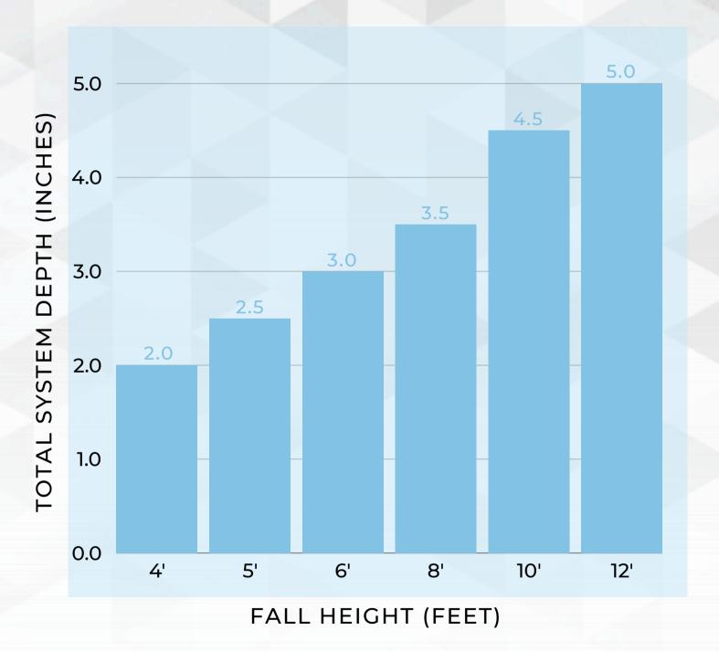
CHART REPRESENTS THE TOTAL (SBR CUSHION & TPV WEAR COURSE) SYSTEM DEPTH EXAMPLE: 2.0" SYSTEM CONSISTS OF 1.5" SBR CUSHION LAYER AND 1/2" TPV WEAR COURSE
