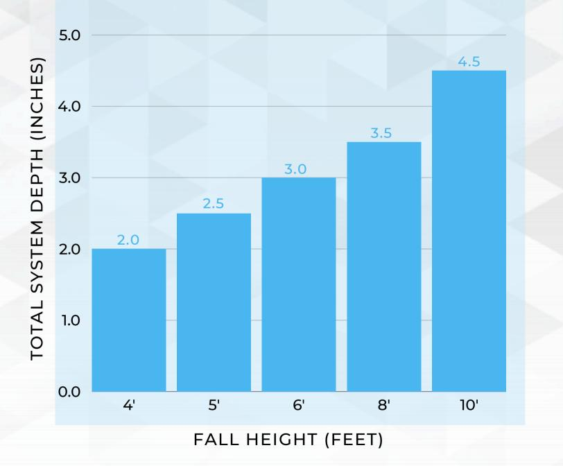
CHART REPRESENTS THE TOTAL (SBR CUSHION & TPV WEAR COURSE) SYSTEM DEPTH EXAMPLE: 2.0" SYSTEM CONSISTS OF 1.5" CUSHION LAYER AND 1/2" TPV WEAR COURSE
